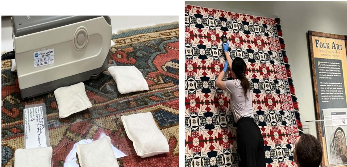
Figure 9. Spectrophotometry of the Turkish rug, stencil mylar templates to facilitate finding the same location twice for accurate readings.
