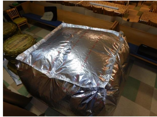
Figure 18: the annoxia bubble constructed and filled with gas is left for 6 weeks
