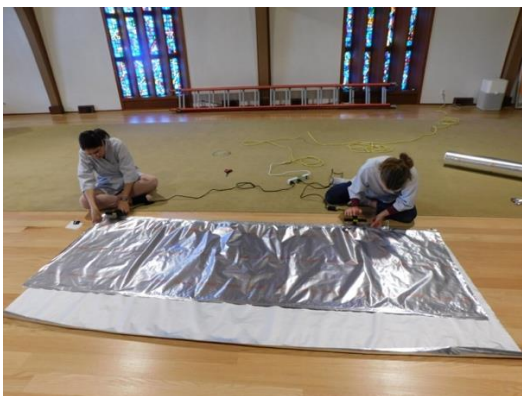
Figure 15: Measuring out pieces of Marvelseal in situ.
