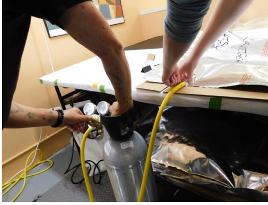
Figure 11: After inserting the object and sealing final seam, as much air as possible has been removed – CO 2 is fed through the unsealed inlet.
