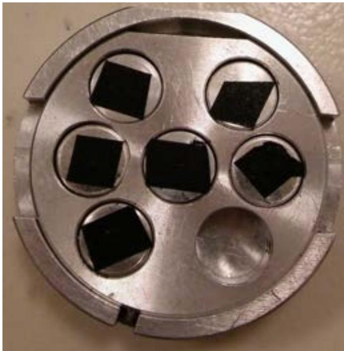
**Figure 16.** The stage on which samples are placed for SEM-EDX analysis. Here the stubs have double-sided carbon tape on them, onto which a sample embedded in resin can be placed, or pinpoint samples of fresh tube paint.
