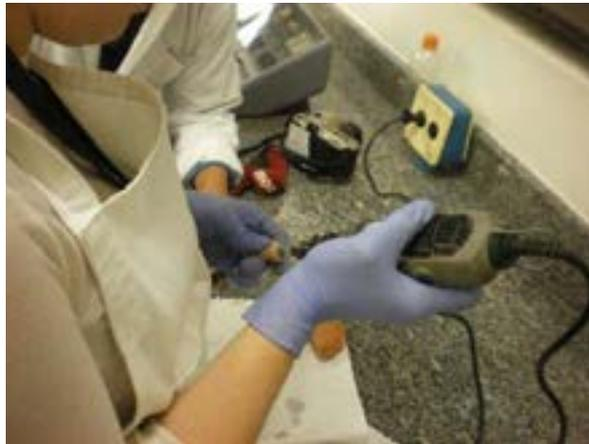
Figure 15. Drilling holes for the armature with a Dremel
