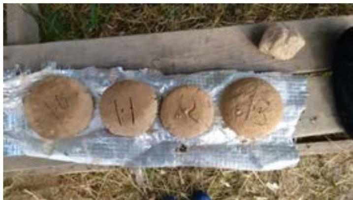
Figure 17. Testing different proportions of soil mixes
