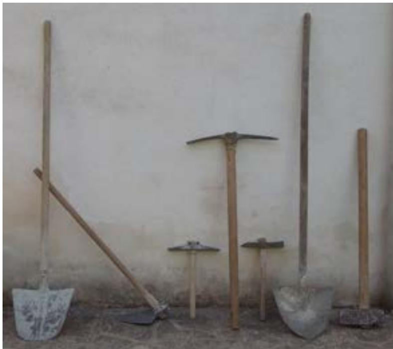
With the exception of a bucket and ladders, these are all the hand tools required for rebuilding a trullo roof. The main tool, a 'trullaro hammer' is pictured third from the right.
