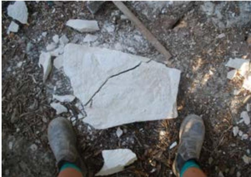
Not to plan: when the limestone splits along a weakness. If the piece was large enough then two smaller chianche could be made.
