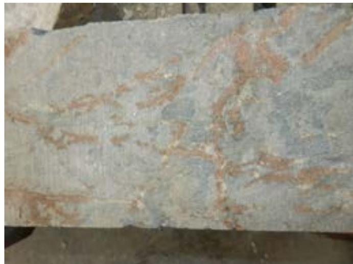
*Figure 25: Stone showing the glue used to secure repair*
