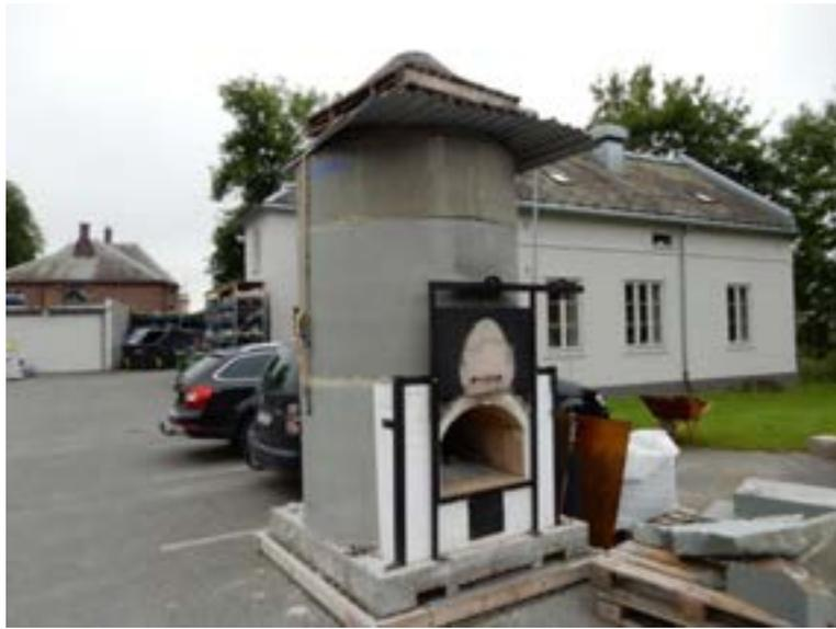
*Figure 32: Kiln used to burn the quicklime*
