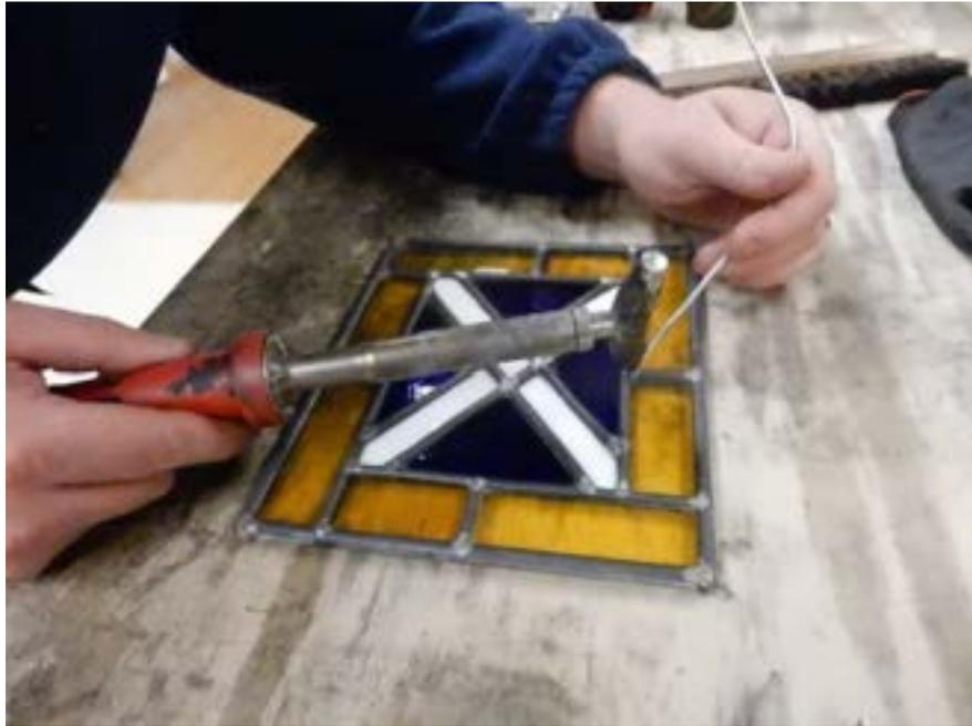
*Figure 40: Soldering the glass together*
