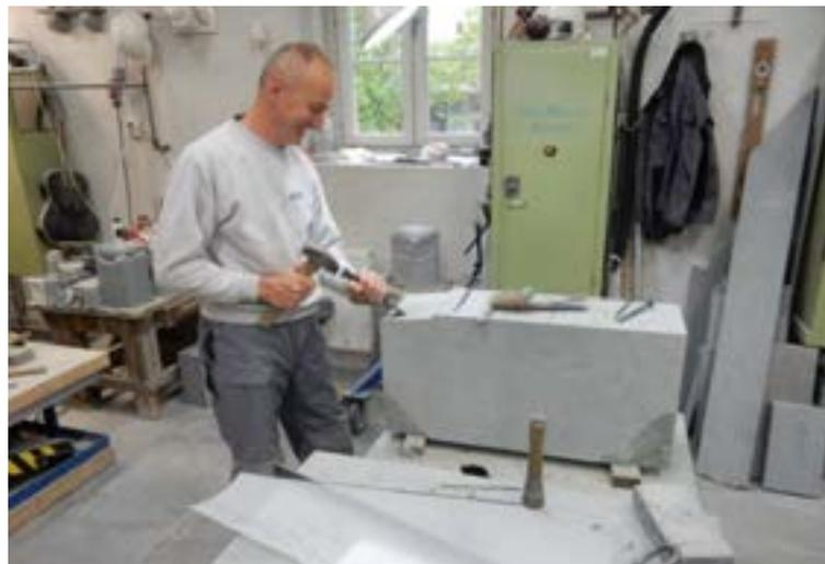
*Figure 15: Roughing out of the stone*
