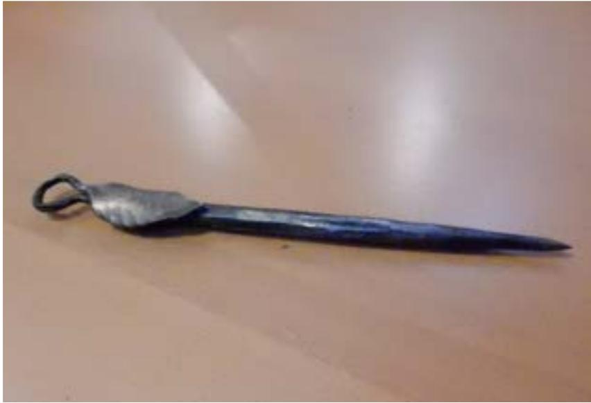
*Figure 48: Finished scribe to mark stones for masonry process*
