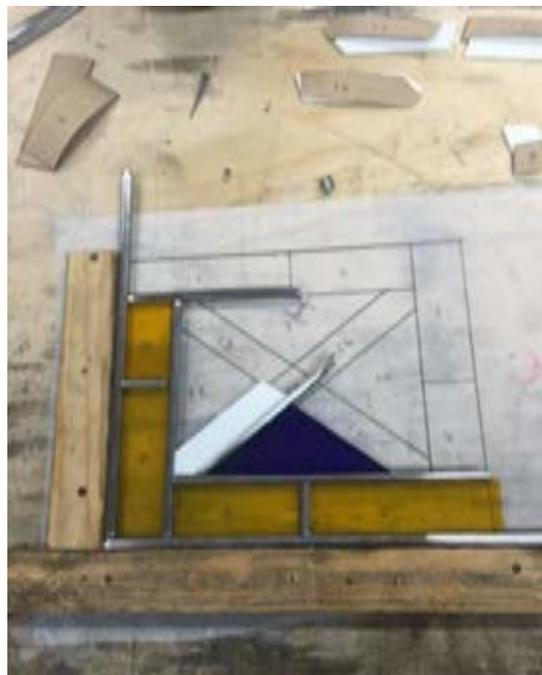
*Figure 39-38: Cutting the glass and laying out the design*
