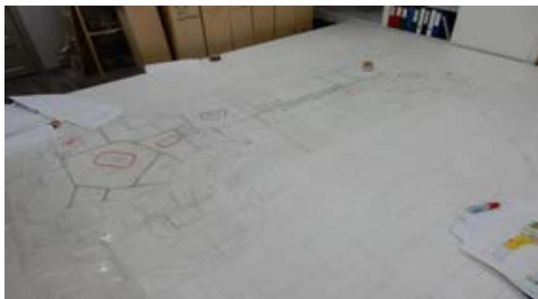
*Figure 13: The tracing floor with full scale drawings*
