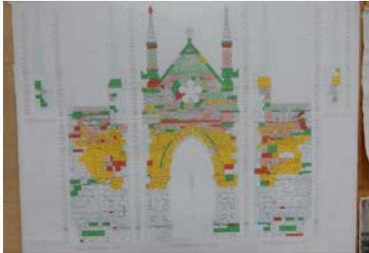
*Figure 12: Marked elevation drawings*
