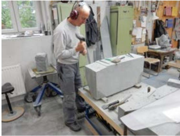
*Figure 16: Trimming off waste with axe*
