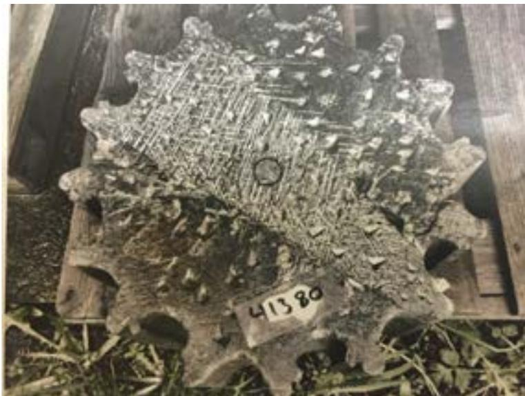
*Figure 21: Repaired stone with dovetail joints*
