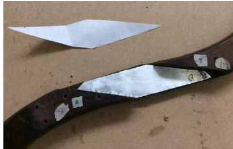
A half assembled joint with the aluminium in situ.
