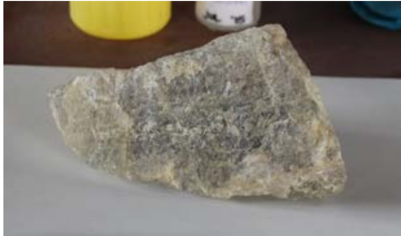
Figure 19. The quartzite stone with a fumed silica and Paraloid B44 fill complete. It was very difficult to have the fill match the transparency and texture of the quartzite stone but after many attempts a good result was achieved. Photograph by A. Duckor
